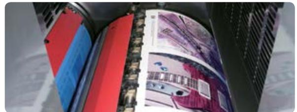
*On the central impression cylinder, sheets are inked with all four colors without gripper changes. Precise registration, from the first sheet to the last, is an inherent feature of the Presstek 52DI and Presstek 52DI ECO-UV press design.*
